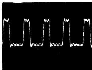
A21J6 .05 usec/DIV .05 volts/DIV 10:1 probe (ac coupled)
